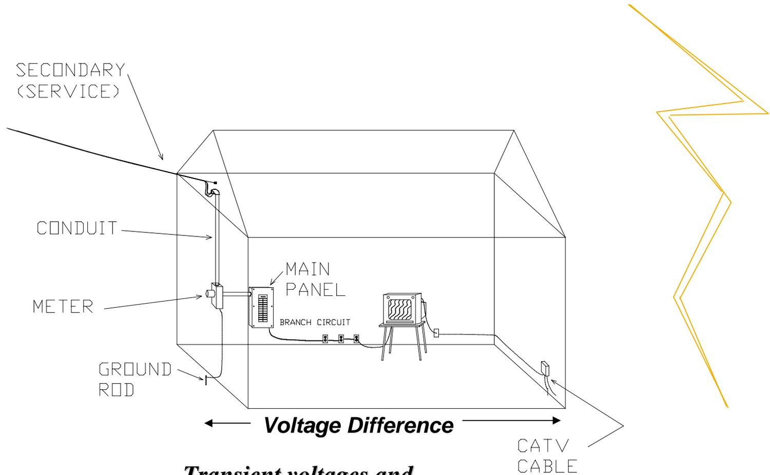
*Transient voltages and currents at data port or cable connections*
